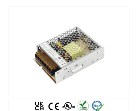
The 56YEL100-x Series is a performance-focused 100W Enclosed AC/DC Power Supply. Designed for use in applications such as network equipment and signal distribution hardware. This series is supplied with a Screw Terminal Block input connection and supports input voltages of 90~264V AC 47~63Hz.
